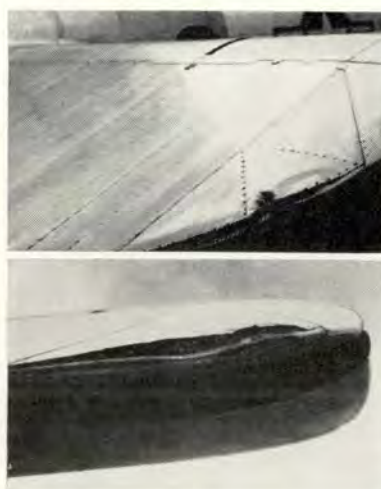
Photos show damage to wing structure as result of lightning discharge. Cockpit overhead window was also smashed.
